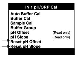
Figure 8-1 Resetting pH Offset and pH Slope
